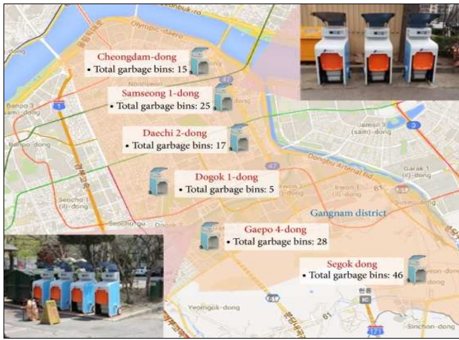
Fig. 1. Locations where SGBs were deployed, their number, and the system implementation
